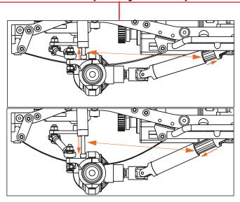
How to insure for proper Driveline phasing.
