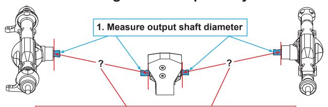
2. Measure distance shown to calculate the proper length driveshaft for your vehicle under full compression and full "Droop" of your suspension.
